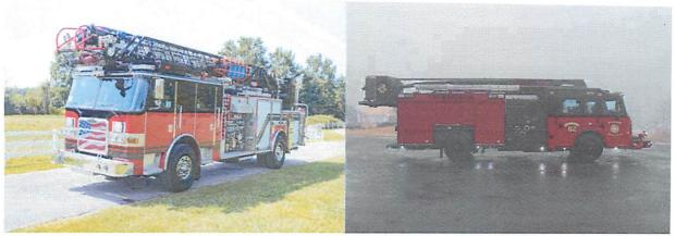
Priority 1 – Ladder 943 – Type 2 Aerial w/75' device with 1,500gpm pump \$425-950,000 project
